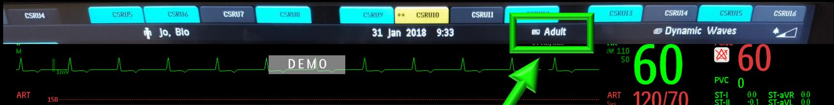
A **PROFILE** (green boxes) is default set of parameters that defines the colors, configuration and alarm limits for all measurements.
