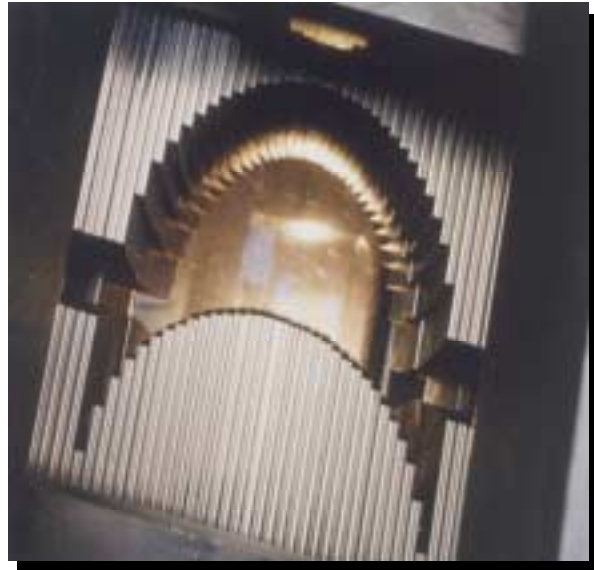
Figure 3. A multileaf collimator (MLC) on an Elekta linear accelerator (looking from the patient's perspective towards the radiation source).
