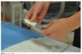
Figure 4: Connect Microsensor™ (white) to Codman Express cable (grey)
