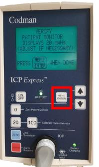
Figure 22: Confirm calibration and select "Menu"
