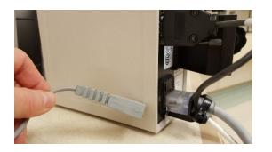
Figure 11: The monitor cable should remain attached to the back of the Codman Express
