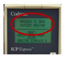
Figure 18: This prompt tells you to select the zero on the pressure module
