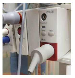
The Philips<sup>TM</sup> end of the Codman Express<sup>TM</sup> cable should be permanently attached to the back of the monitor (Figure 12).
