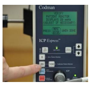
Figure 21: Send calibration signal "20" to the Philips monitor.
