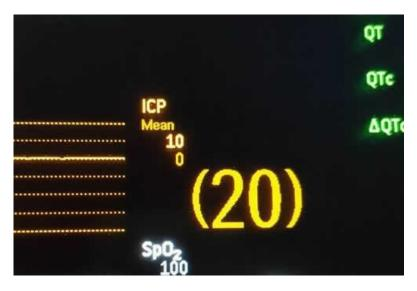
Figure 22: When pressure reaches 20, calibration has been achieved.
