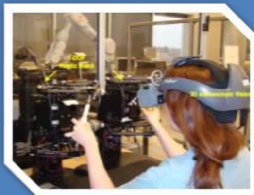
Leader-follower teleoperation for haptics-enabled robotics assisted surgery
