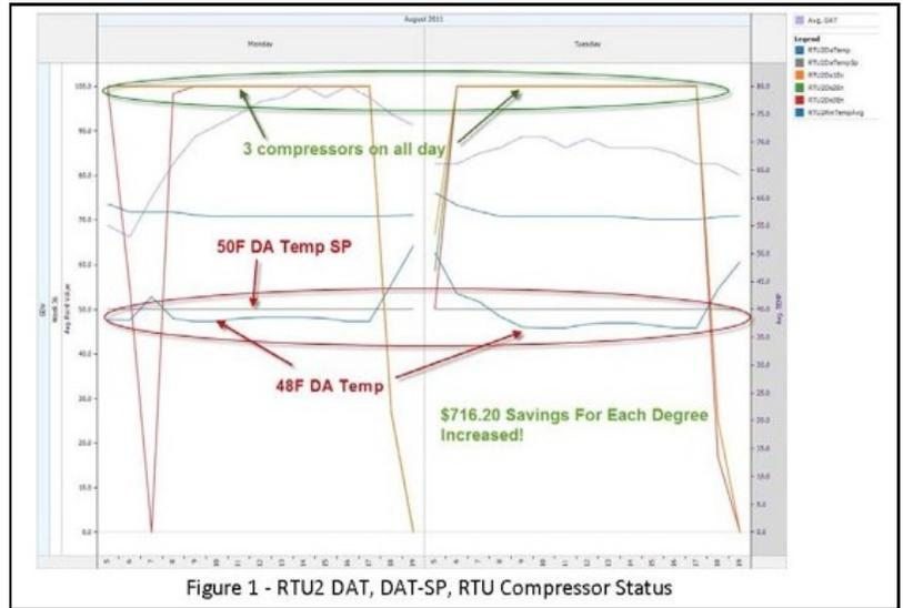
Figure 1 - RTU2 DAT, DAT-SP, RTU Compressor Status
