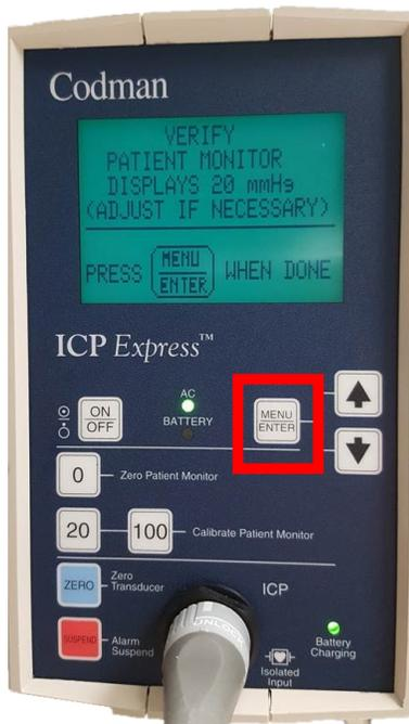
**Figure 22: Confirm calibration and select "Menu"**
