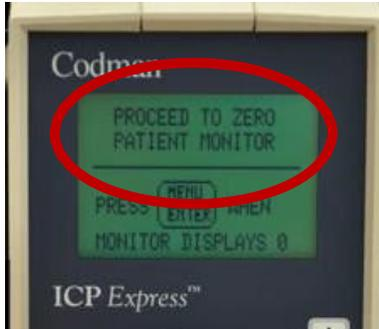
**Figure 18:** This prompt tells you to select the zero on the pressure module
