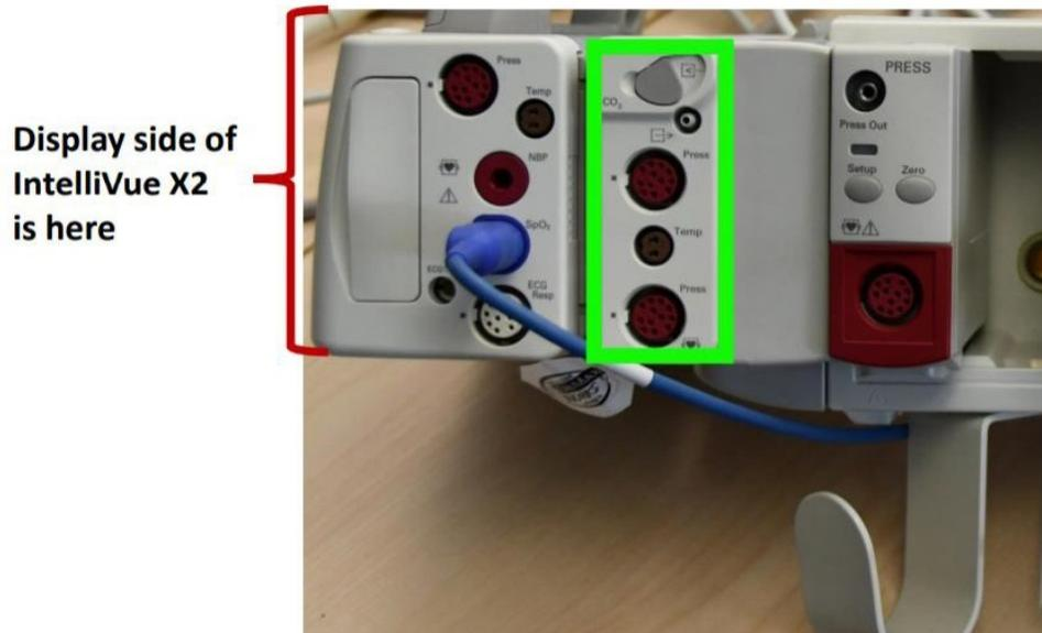
Figure 10: Identify a spare module
