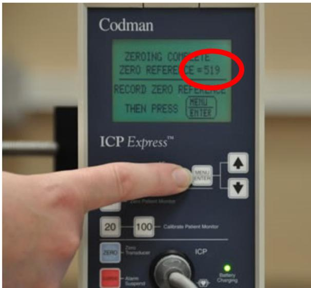
**Figure 9: Identify reference code and complete zeroing**
