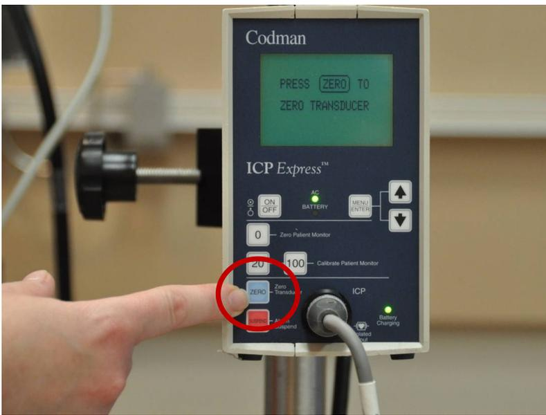
**Figure 8: Press blue “Zero Transducer” button. ONLY EVER SELECTED DURING INSERTION**
