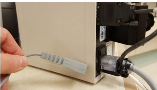
Figure 11: The monitor cable should remain attached to the back of the Codman Express
