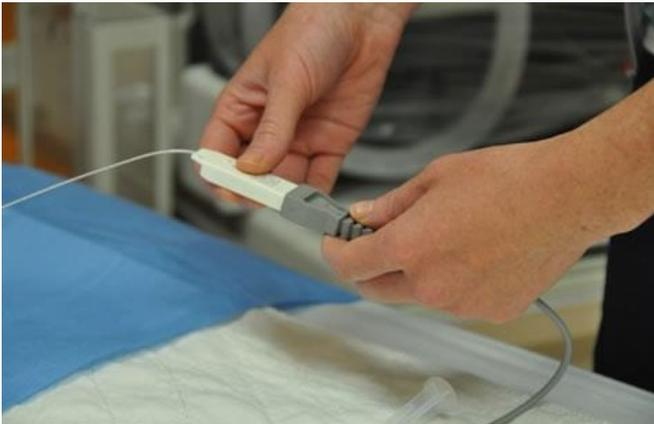
**Figure 4:** Connect Microsensor™ (white) to Codman Express cable (grey)
