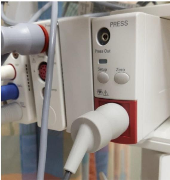
**Figure 12:** Philips™ end of the ICP monitoring cable plugged into single module. The pressure cable has a different coloured connection (white) than other Philips cables (grey).
