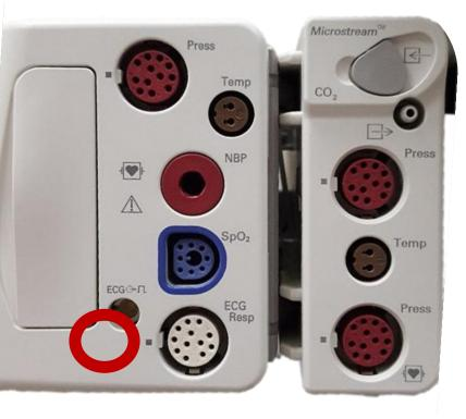
The synchronization INPUT jack on the IntelliVue X 2 is available if you wanted to bring an ECG from another source to the IntelliVue X2 or monitor.
