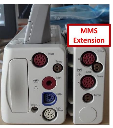
The IntelliVue X2 is mounted to the rack by attaching it to a "Measurement Extension" (called an MMS extension).
