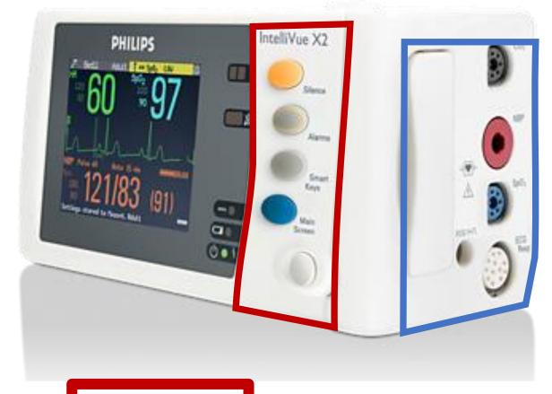
Each IntelliVue X2 includes ECG, one pressure, NIBP, temperature and SPO2 cables are connected at the side.
