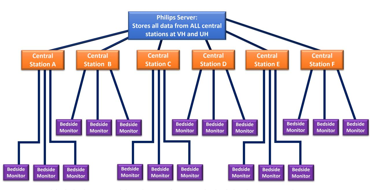
From each bedside, data is routed through a central station and uploaded to the main network server. Monitoring data can subsequently be transferred from the network to any bedside monitor with 7 days of admission.
