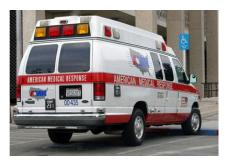
c) Type III: van chassis with an integrated modular box on the back for medical care and equipment
